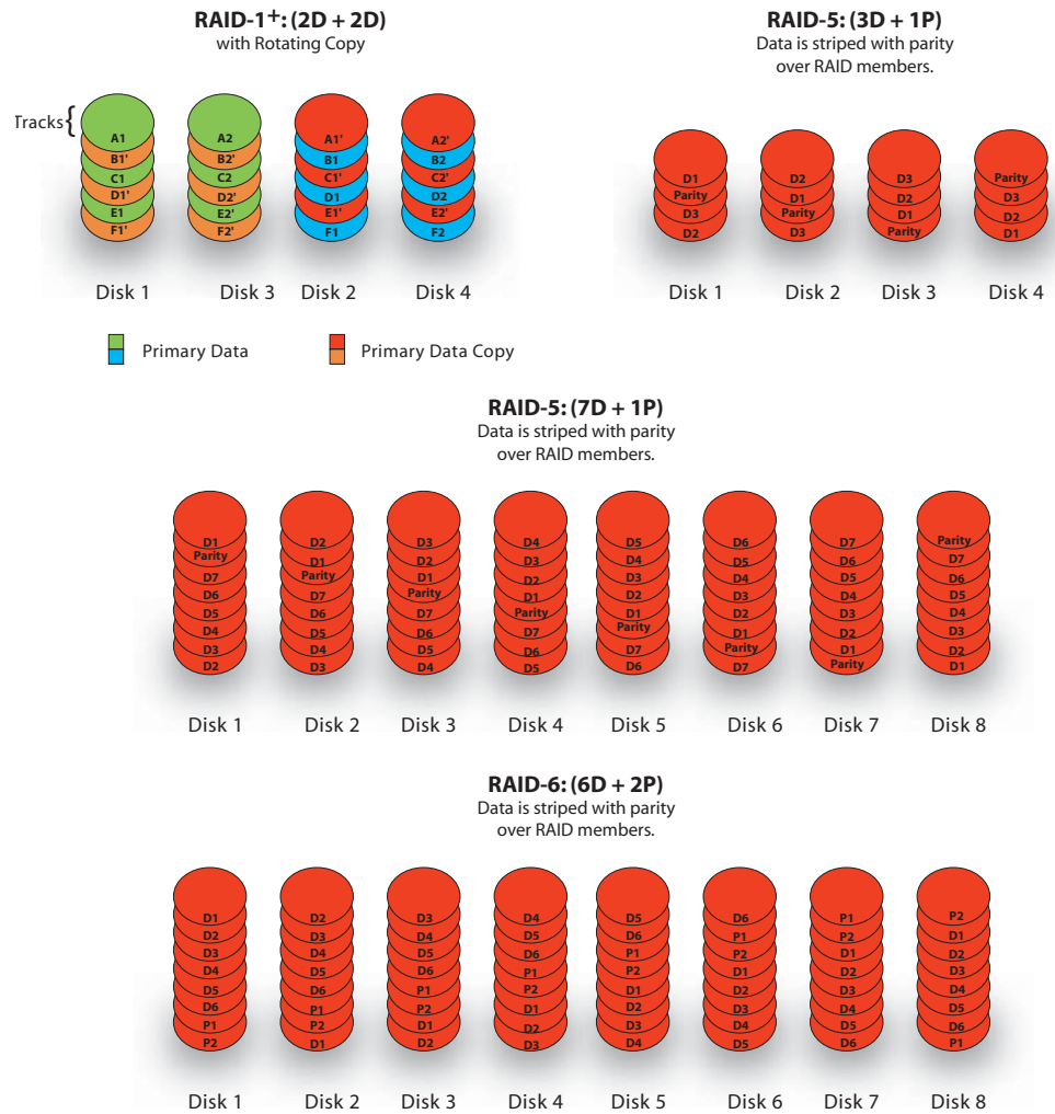
Figure 24. All Universal Storage Platform and Network Storage Controller models are available with RAID-1+, RAID-5, and/or RAID-6.
